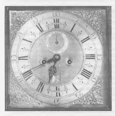
The illustration on the left is of a face of a long-case clock made by Richard Lloyd of Cowbridge in the early eighteenth century. It is an eight-day movement, striking the hours, in an oak case. The dial is brass, with a silvered chapter ring. Some of the detailed features of the clock suggest a date of between 1725 and 1740.
