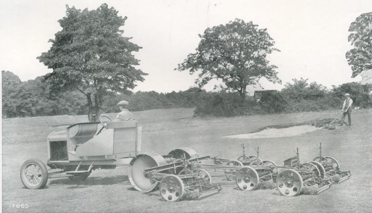
TRACTOR AND QUINTUPLE MOWER (CAPACITY 7 ACRES PER HOUR) OPERATING ON A GOLF COURSE
