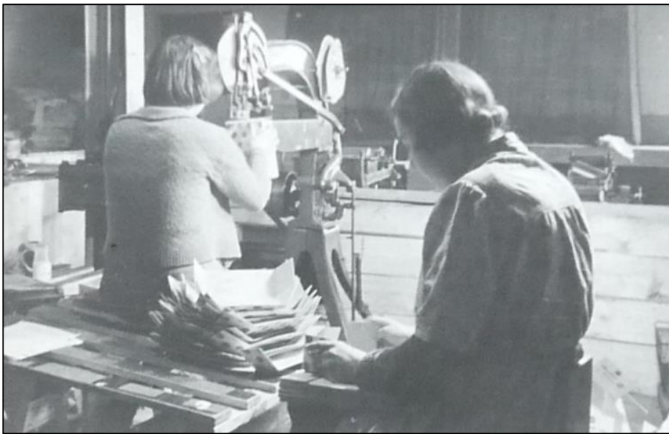
Workers at the General Paper and Box Manufacturing Company reinforcing the corners of pre-folded boxes.
